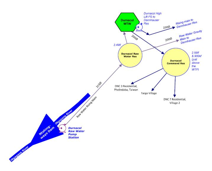
Figure 14.35 Durnacol WTP Supply Schematic (not to scale; Amajuba DM Water bulk infrastructure)
