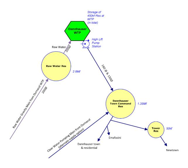
Figure 14.32 Dannhauser WTP Supply Schematic (not to scale; Amajuba DM Water bulk infrastructure)
