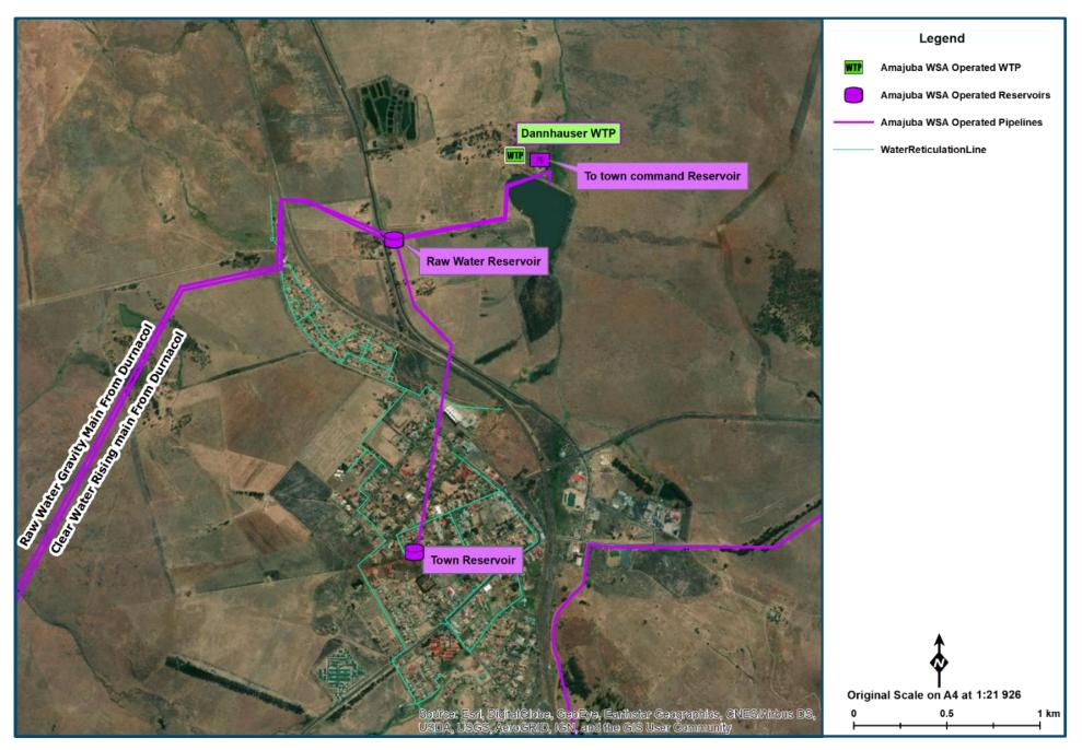
Figure 14.33 Dannhauser Supply System Layout (Dannhauser WTP System) (NGI 2014; Umgeni Water 2020)
