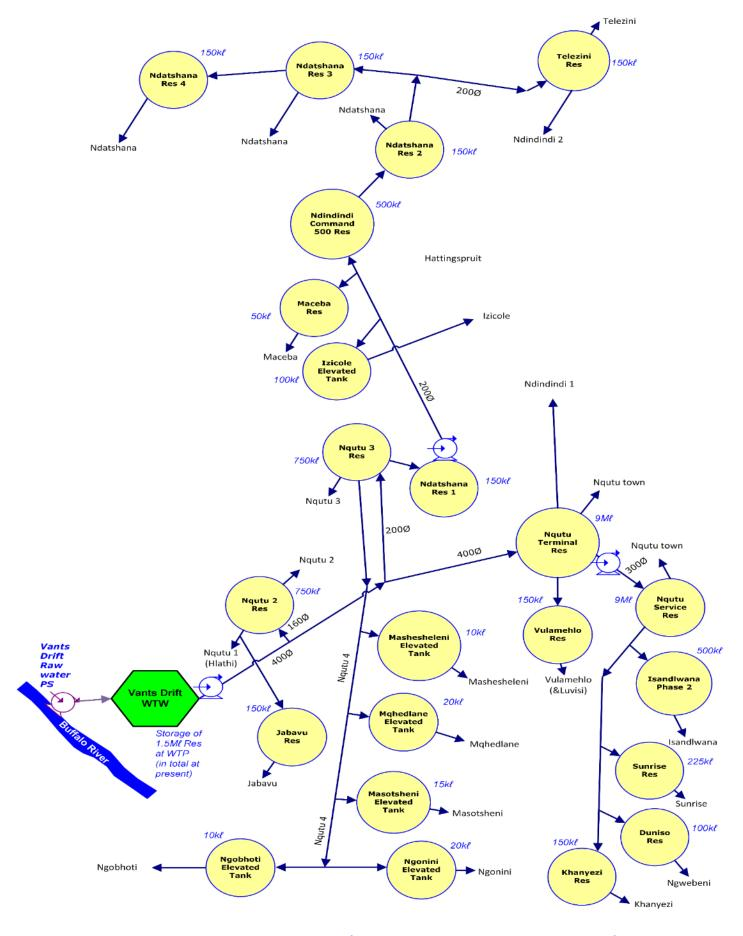
Figure 14.30 Vants Drift WTP Supply Schematic (not to scale; uMzinyathi DM infrastructure)
