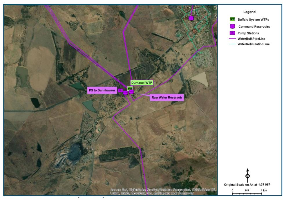
Figure 14.36 Durnacol Supply System Layout (Durnacol WTP System) (NGI 2014; Umgeni Water 2020)
