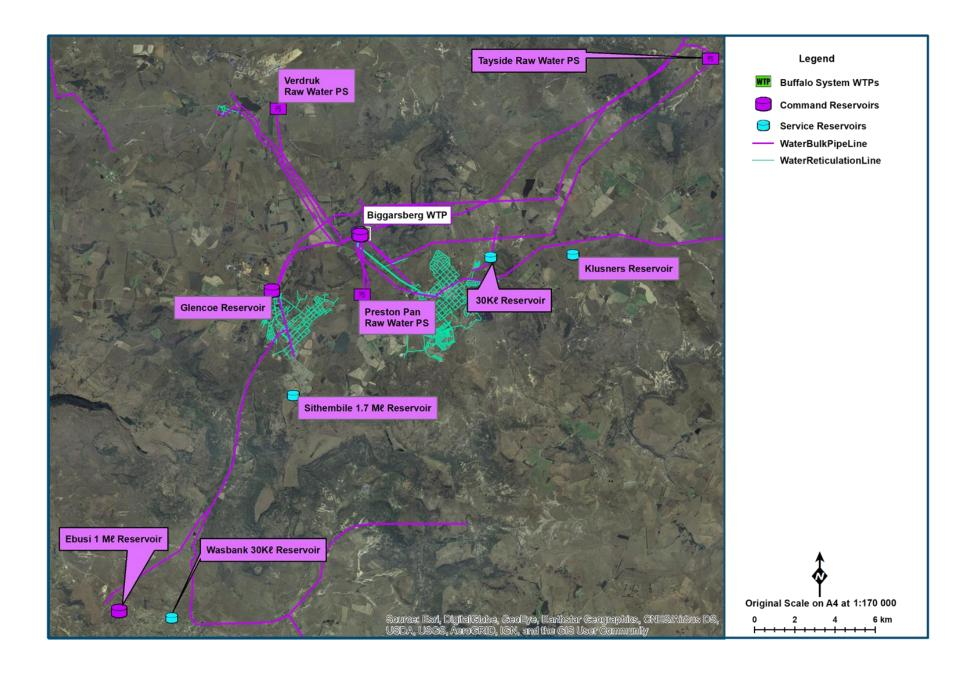
Figure 14.27 Dundee/Glencoe Supply System Layout (Biggarsberg WTP System) (NGI 2014; Umgeni Water 2020)
