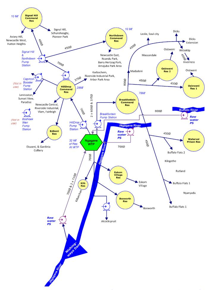
Figure 14.21 Ngagane WTP Supply System Schematic (not to scale; uThukela Water bulk infrastructure)
