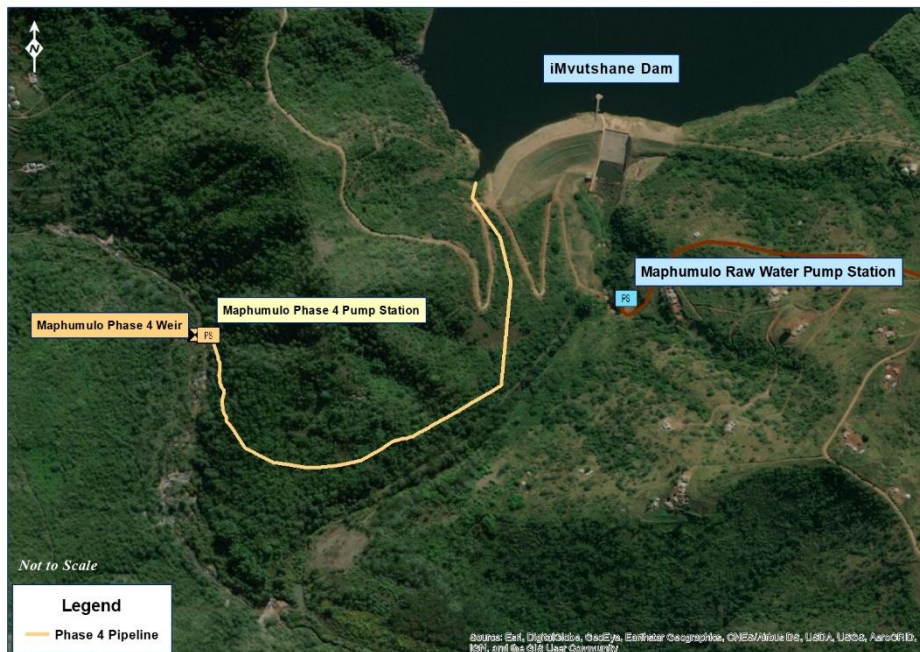
Figure 12.13 Locality map showing the proposed Hlimbitwa River weir pump station in relation to iMvutshane Dam.
